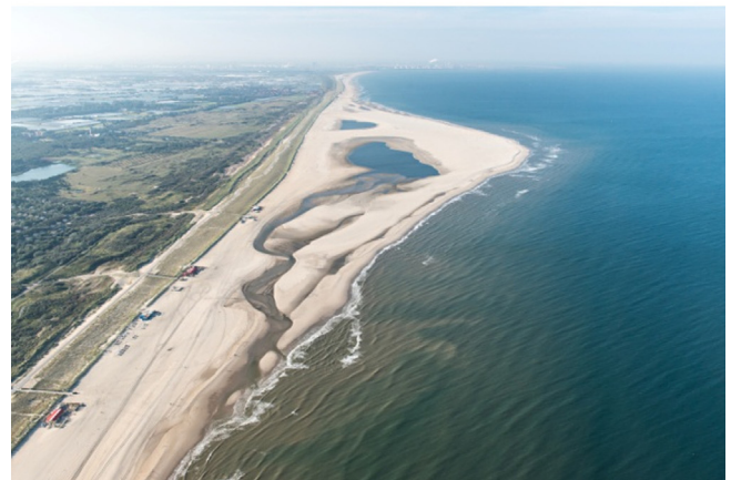
Fig. 8. Upper panel: The Delfland Sand Engine shortly after placement (July 2011). Lower panel: The Sand Engine has evolved into an almost symmetrical salient (October 2013). source: https://beeldbank.rws.nl , Rijkswaterstaat/Joop van Houdt.
