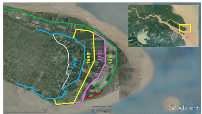
Fig. 17. Consecutive reclamations of accreted marsh on East Chongming Island, Yangtze Estuary, China.
