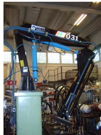
Figure 10. Water hydraulic boom with proportional control valves [8].
