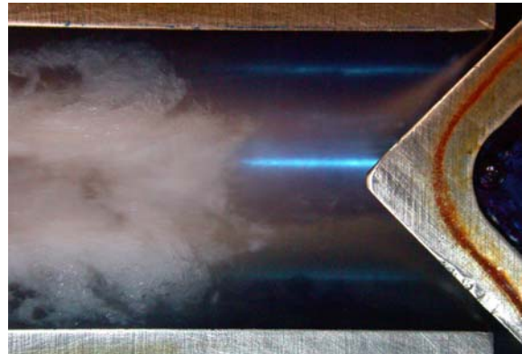
Figure 4. Unsteady situation of cavitating flow.
