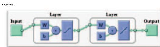
Fig. 8.2 Simplified ANN used with several inputs, hidden neurons with coefficient arrays ( W and bias b ), and outputs
