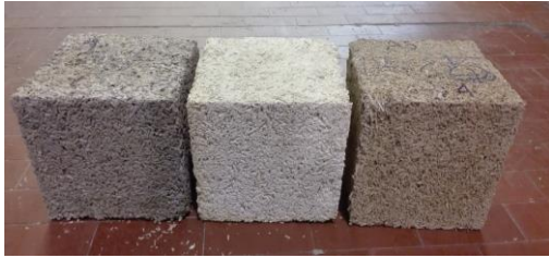
Figure 2. Hempcrete samples of three different companies (A3, A4, A5)
