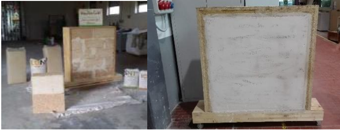
Figure 4. Hempcrete blocks' wall in the framework
