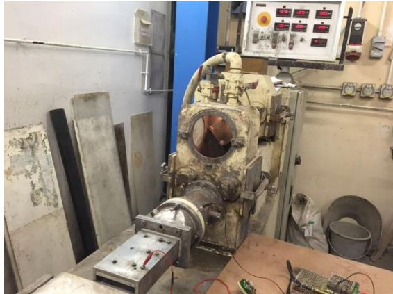
Fig 3.3 Extruder (PVL100.3, KEMA)
