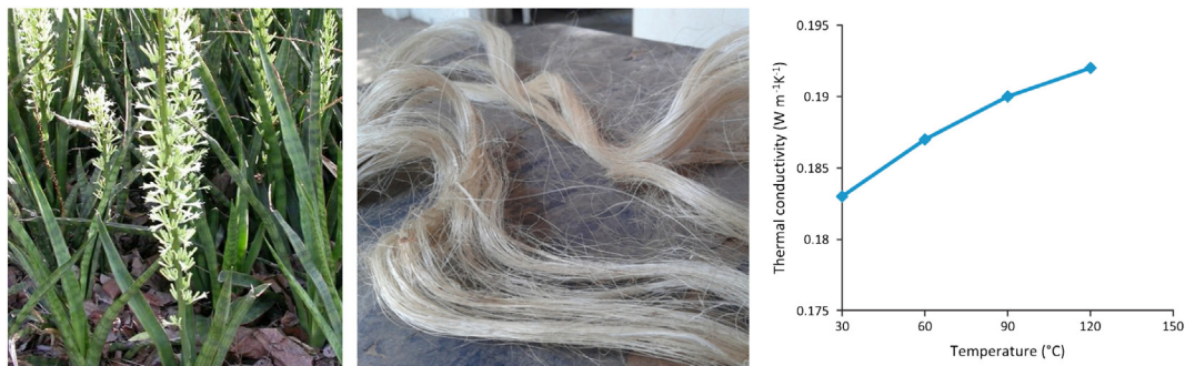
Fig. 13. Sansevieria plant (left) and fiber (middle). On the right, thermal conductivity trend vs. temperature measured in [78].
