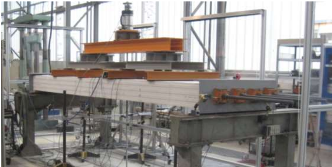
Figure 5: Test set-up for bending
