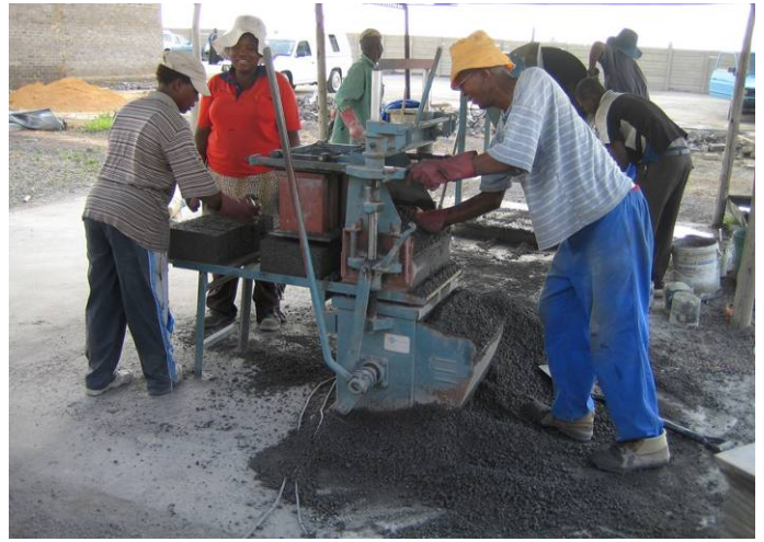
Figure 5. Production of local scoria and cement bricks
